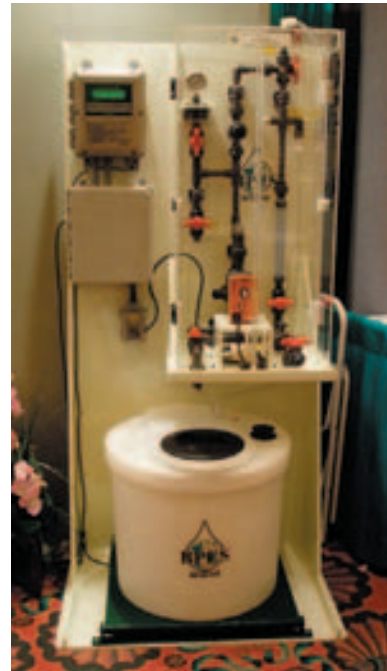
IS system with full featured electronic scale indicator and electronic metering pump.
