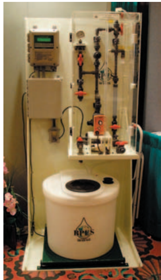
HFS system with full featured electronic scale indicator and manual electronic metering pump for remote on/off control.
